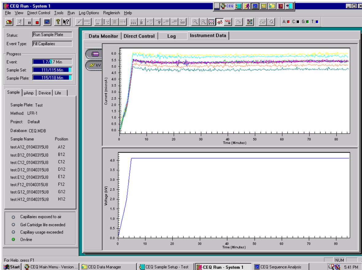
**Figure 42: Viewing the Instrument Data Window - Current and Voltage**
