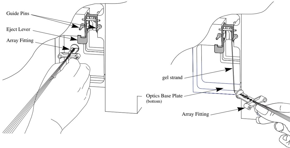
**Figure 10: Cleaning the Detection Window**
