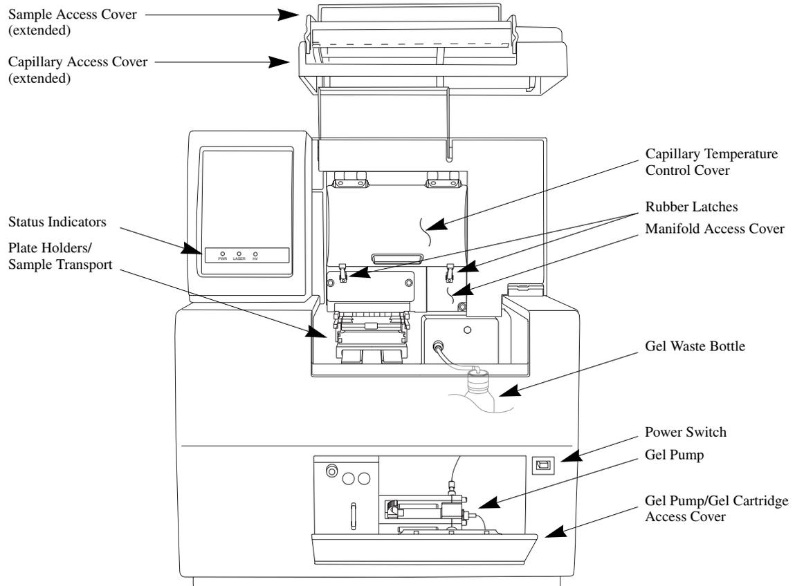
**Figure 4: User Accessible Hardware Components**
