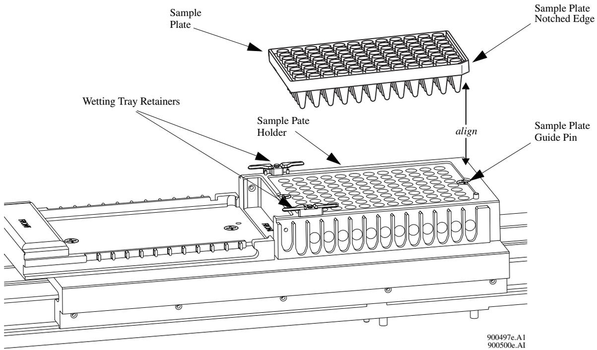
6. When finished positioning the plate, close the Sample Access Cover and then click the **Load** button of the **Capillaries Exposed** dialog box (Figure 39).
