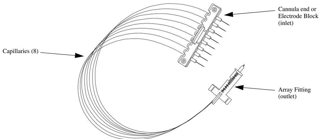
Figure 5: Capillary Array
