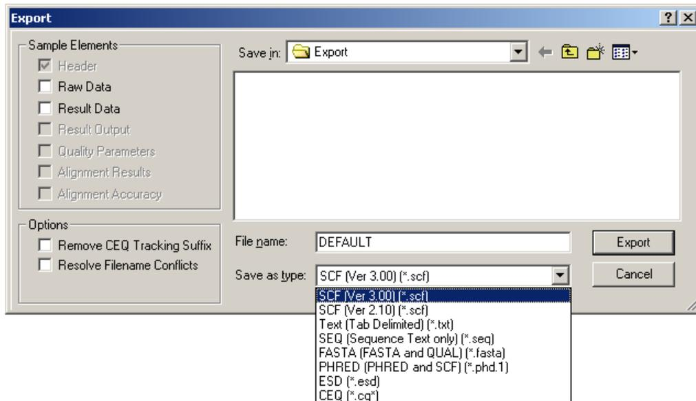
4. Select the file type. Some sample elements are grayed-out, or automatically checked when the different file types are selected. If the element is grayed-out and unchecked, the option is not available for that file type. If the element is grayed-out and checked, that item is automatically exported. These options differ for sequence data and fragment data.
