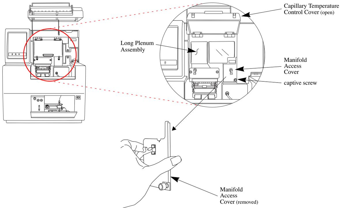
**Figure 9: Manifold Access Cover**
