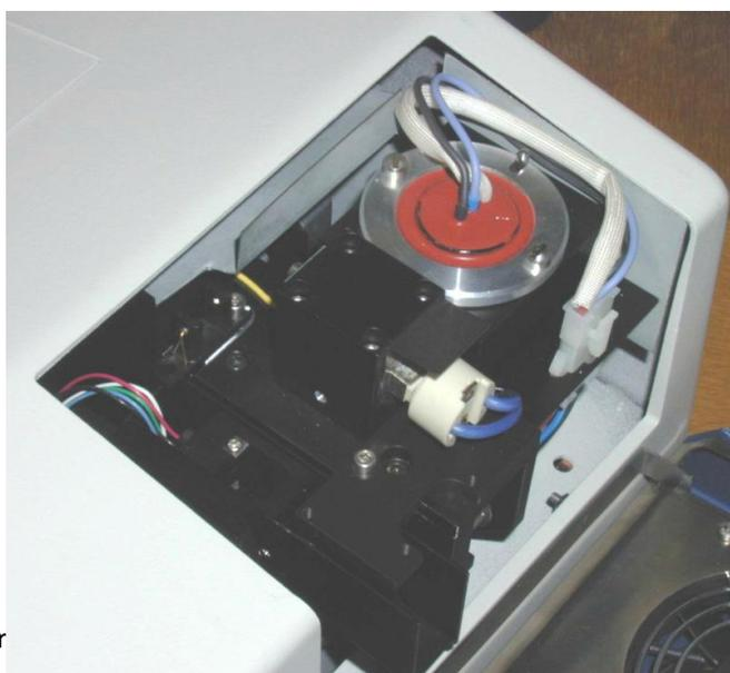
5. Remove the two flathead screws that secure the deuterium lamp (Figure 3-4).
