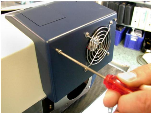
Figure 3-2. Removing the allen screws
