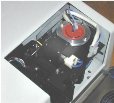
Figure 3-6. Halogen lamp and lamp block assembly
