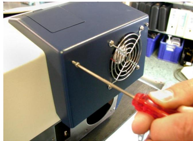
Figure 3-5. Removing the Allen screws
