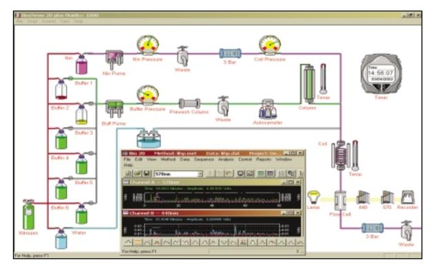
The system is operated via an advanced graphical user interface which shows the instruments operational information in real time and is fully integrated with the data-handling software.
